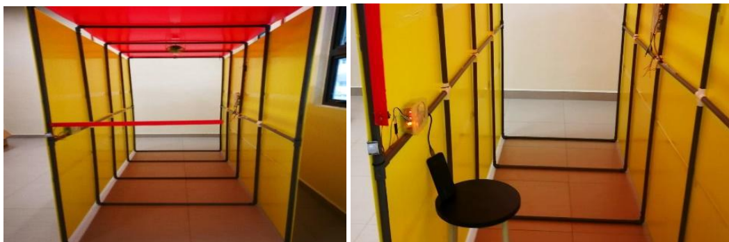
Figure 10. The smart home design (left). The door open when PIR sensor detects any motion in front of the door (right)
