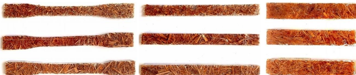
Fig. 2. Tensile Test Specimen; Fig. 3. Flexural Test Specimen; Fig. 4. Impact Test Specimen
