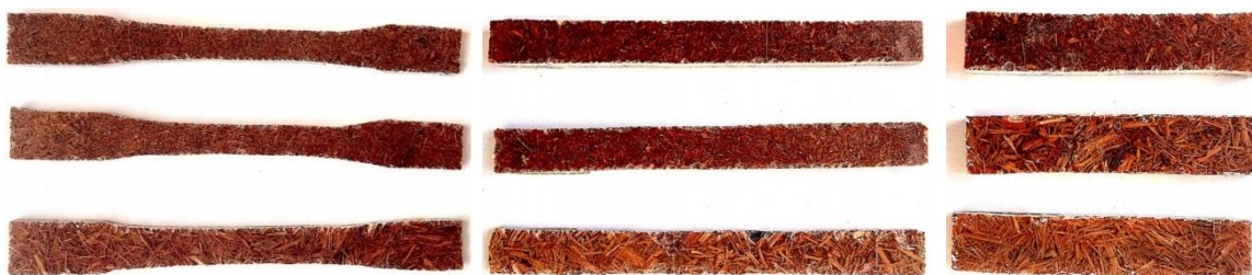
Fig. 5. Tensile Test Specimen
