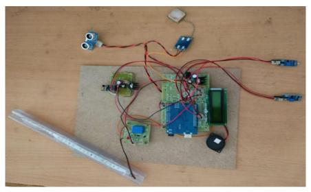
The above image shows the hardware equipment of the project. The kit is turned ON by giving the regulated power supply of 12v which is then converted to 5v dc current. The generated 5v dc current passes to every hardware component in the circuit.
