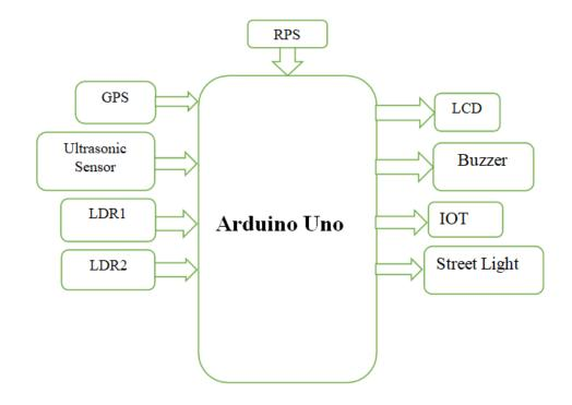
The proposed IoT-based system for manhole monitoring and street light control with fault detection and reporting capabilities represents a cutting-edge solution for municipalities to efficiently manage their infrastructure.
