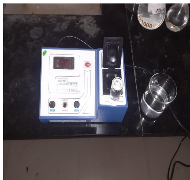
Fig. 1. Turbidimeter set-up to test turbidity for both the groups of water samples. A total of twenty iterations of the turbidity measurements were taken to avoid discrepancies
