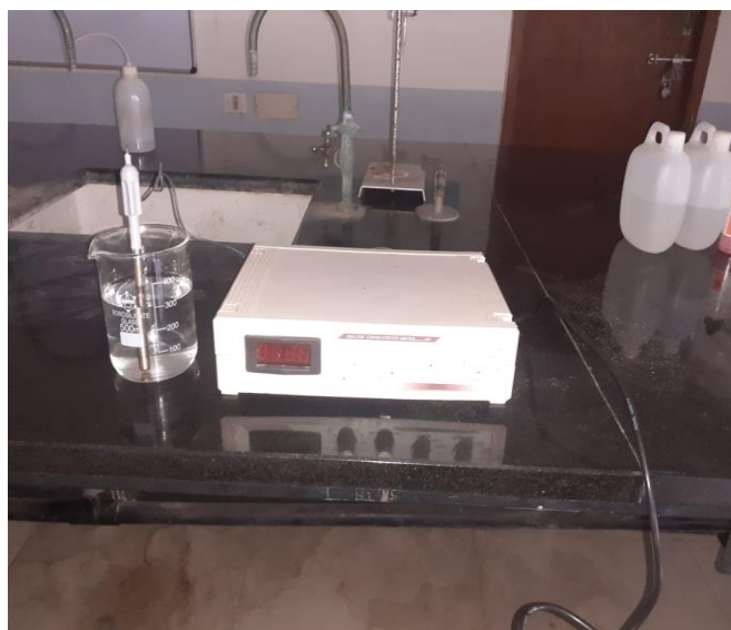
Fig. 2. Electrical conductivimeter setup with electrolyte for testing EC in both groups of water samples. Twenty numbers of iterations were taken and averaged to obtain the EC values.
