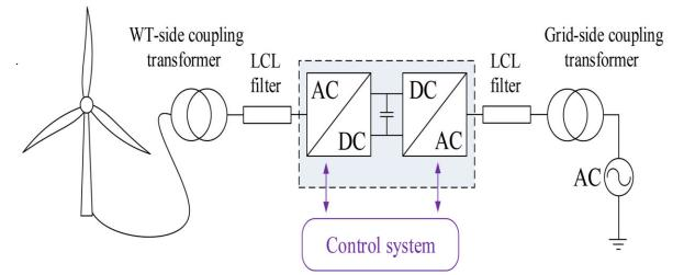
This structure has back-to-back connected converters of wire turbine with permanent magnet synchronous generator (PMSG), both these are connected to same bus with loads. The loads are combination of linear and highly inductive loads causing harmonics at the PCC (point of common coupling).
