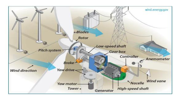
Wind power is generated by wind power plants. It consists of wind blades, wind turbine, double fed induction generator which converts wind energy into electrical energy.
