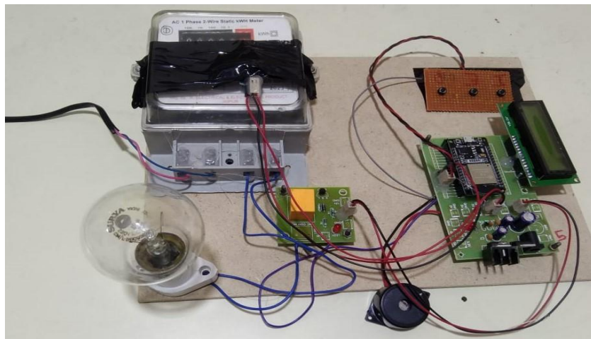
Figure 3. IOT based energy consumption meter
