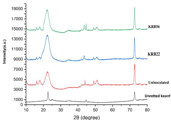
Fig. 7. XRD spectra of bacterial, uninoculated and un retted raw kenaf fiber
