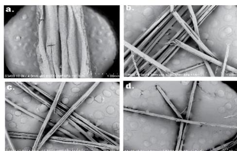
**Fig. 5.** SEM view at 100mm magnification showed the individual kenaf fibres sizes image a. showing higher width sizes of intact raw kenaf fibre before retting b. after retting by un inoculated bacterial strains possess comparably higher diameters indicates the presences of gums and c. retted with *Bacillus* sp. KRB22 and d. *Bacillus* sp. KRB56.
